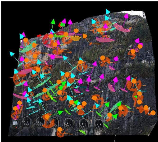
Fig. 3. Screen capture showing the Sirovision 3-D photogrammetric model with 109 mapped rock mass discontinuities. Colors correspond to the sets listed in Table 1 and the arrows represent the normals to the discontinuities.
