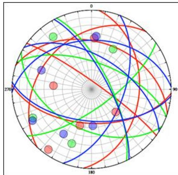
Fig. 6. Equal area polar projection displaying the combined poles with great circles from the different mapping areas [7].
