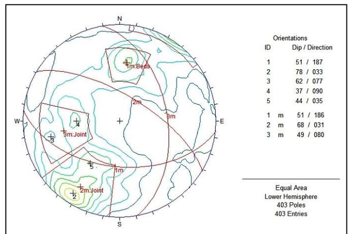
Fig. 7. Equal area equatorial projection of combined discontinuity poles and sets (represented as "m").
