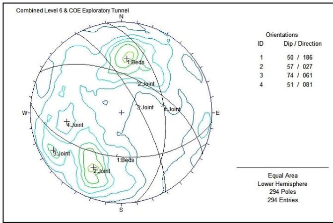
Fig. 4: Combined Level 6 and COE exploratory tunnel equal area stereonet.
