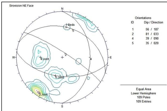
Fig. 5. Equal area stereonet using Sirovision for the northeast face of the rock massif.
