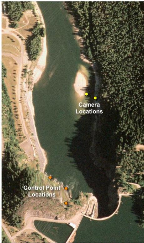
Fig. 2. Orthophoto showing Boundary Dam and its forebay, the Pend Oreille River, the dolomite massif, and the camera locations and control points used for photogrammetric modeling. North is towards the top of the photograph.
