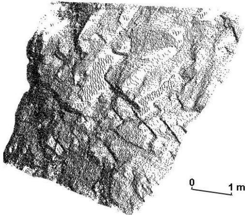
Figure 4. Example 3D point cloud of blocky rock face of the Tremough road cutting, created using laser scanning and subsequently used in Split FX
