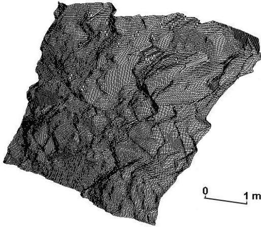
Figure 3. Example 3D mesh of blocky rock face of the Tremough road cutting, created using Sirovision.
