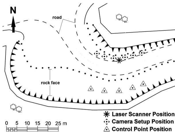
Figure 1. Schematic plan of the Tremough Campus Entrance, showing camera, laser scanner and control locations.
