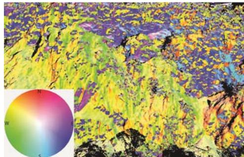
Figure 7. Example of the orientation hillshade created based on the terrestrial LiDAR data for the Wakefield Terrace fieldsite.
