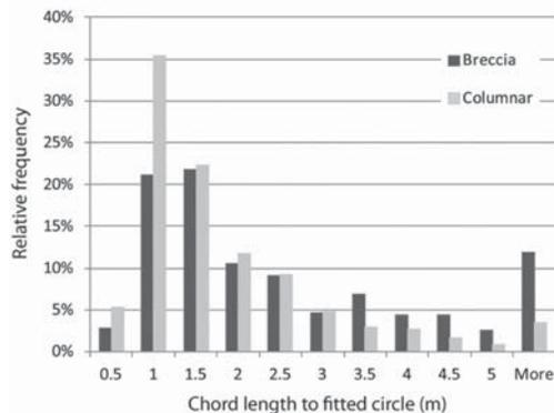
Figure 11. Relative frequency of discontinuity the trace lengths observed in the two geological units based on the terrestrial photogrammetry results.
