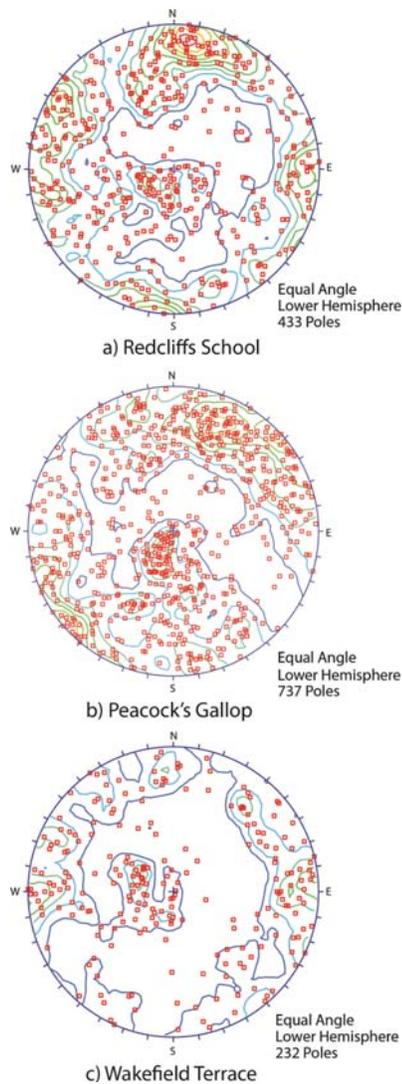
Figure 8. Stereographic projection of the poles to the discontinuities measured in the 3D models for a) Redcliffs School, b) Peacock's Gallop, and c) Wakefield Terrace.
