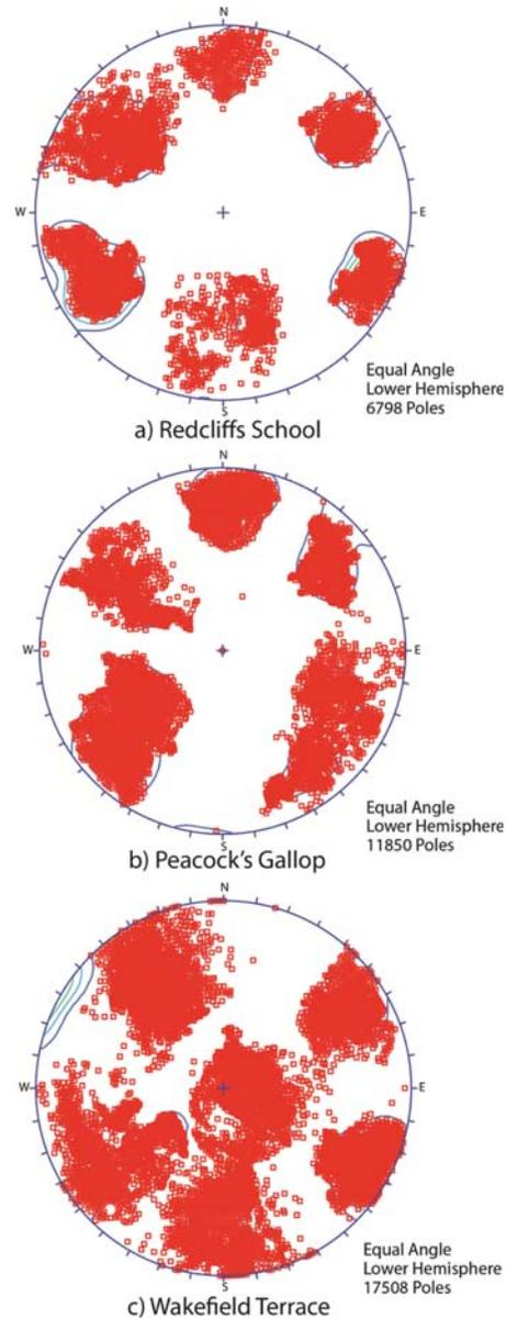
Figure 9. Stereographic projection of the poles to the planar surfaces measured using the terrestrial LiDAR dataset and the software COLTOP for a) Redcliffs School, b) Peacock's Gallop, and c) Wakefield Terrace.
