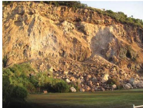
Figure 5. Overview of the geology and rockfall talus at the Wakefield Terrace field site.
