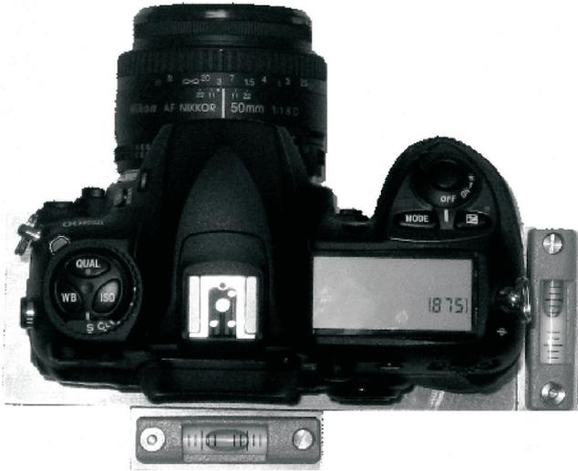
Figure 1: Camera mounted on custom levelling plate
